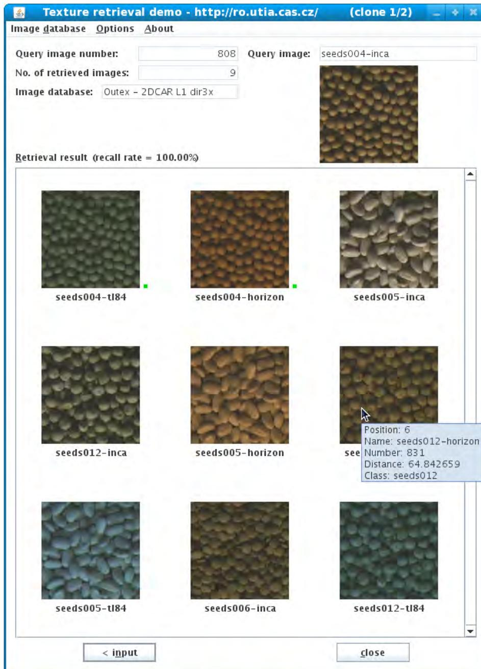
Figure C.4: Result screen of the desktop demonstration. The query image and retrieval parameters are revised in the upper part, while the retrieved images are shown in the rest of the screen. Additional information is provided in tooltips.
